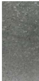
Figure 3 Dull Gray Passivated Zinc
