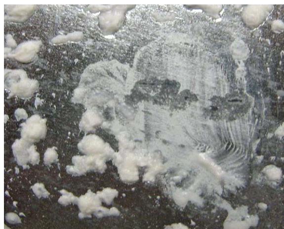
Figure 1 – Waxy White Rust Cells
