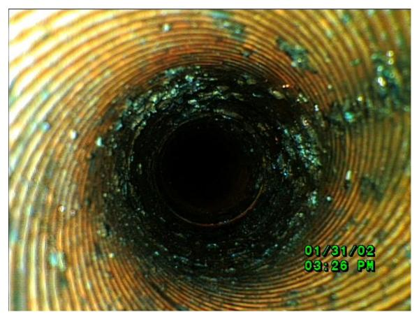
Fiberoptic Scoping reveals severe deposition and corrosion.
