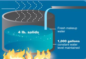
Cycles = Conductivity System Water
